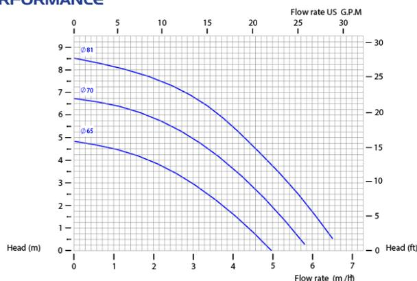
The curves and performance values refer to pumps with free delivery outlet with water at 20 °C, and two poles motor 50 Hz
