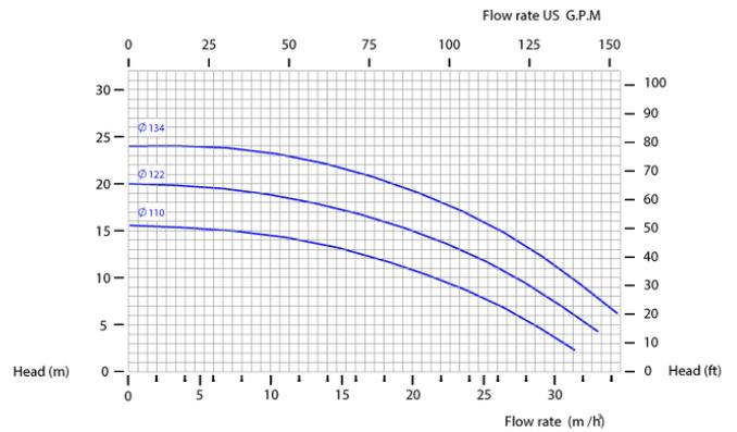
The curves and performance values refer to pumps with free delivery outlet with water at 20 °C, and two poles motor 50 Hz
